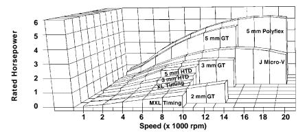
Fig. 5 Horsepower Ratings at High Speed
