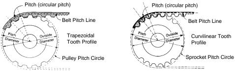
Fig. 1 Pulley and Belt Geometry
