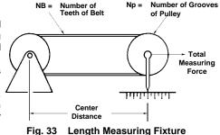
In measuring the length of a synchronous belt, the belt should be rotated at least two revolutions to seat it properly and to divide the tension equally between the two spans.
