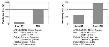
Fig. 10 Comparison of Positioning Errors of Various Belts
