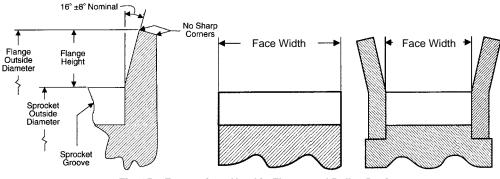
Fig. 35 Expressions Used in Flange and Pulley Design
