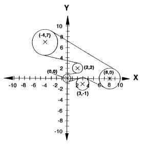
Fig. 28 Example of 5-Point Drive System
