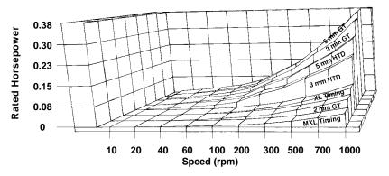
Fig. 6 Horsepower Ratings at Low Speed
