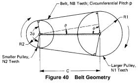
The basic equation for the determination of center distance is:
